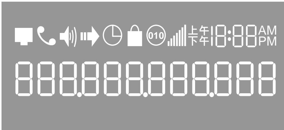
The LCD is equipped with a backlight. When the phone is in the normal idle state, the backlight is off. Whenever an event occurs, the backlight turns on automatically and brings the user's attention.
